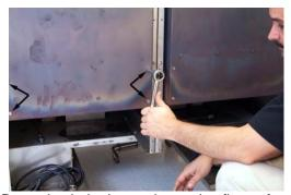
Removing bolts (arrows) securing flue to frypot.
